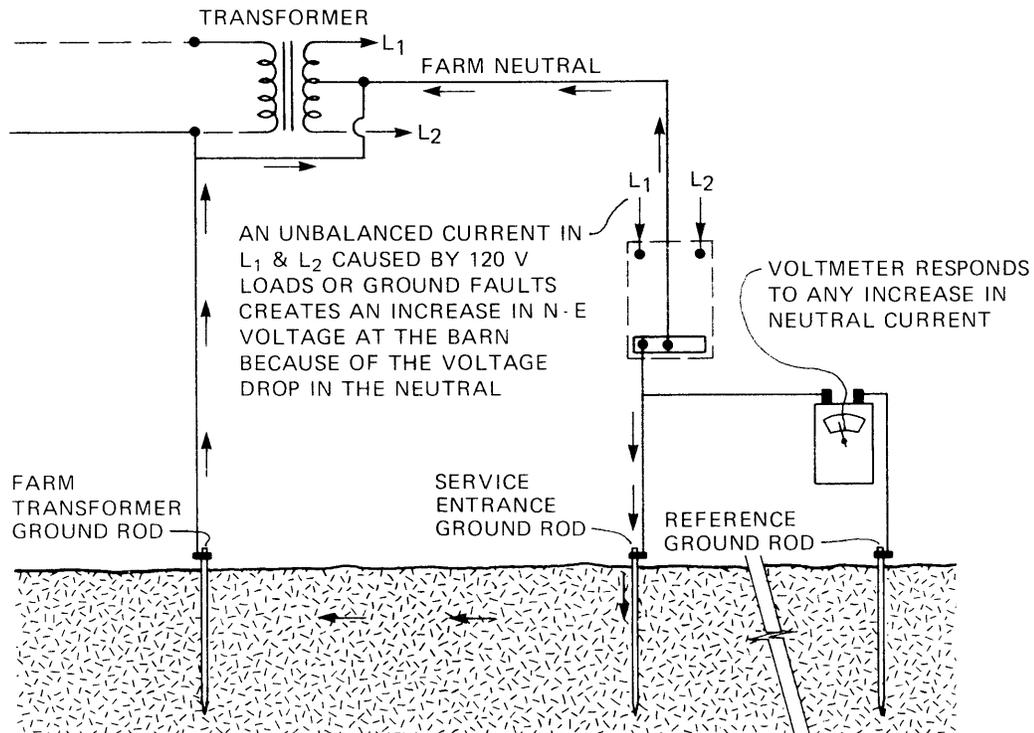
Figure 3 N-E voltages on the secondary neutral resulting from unbalanced 120 V loads
