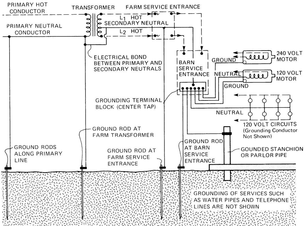
Figure 1 The grounded neutral network on a single-phase primary distribution line and secondary farm service
